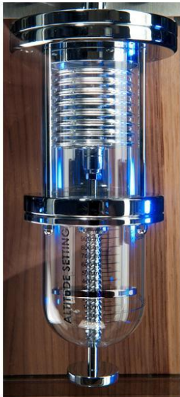
Figure 3: Vacuum metal containers react to the changing air pressure. A combination of 8 vacuum boxes can give an extremely accurate measurement of even the slightest change in pressure.
